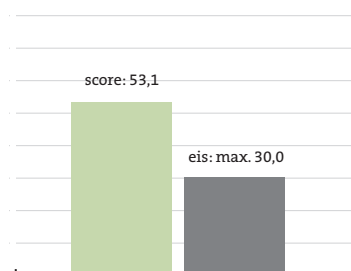
BENG 2: Primair energiegebruik (in kWh/m 2 )
