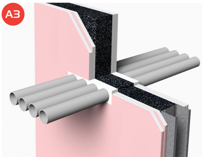
FZ100 Fire Safe Zone and combustible pipes
