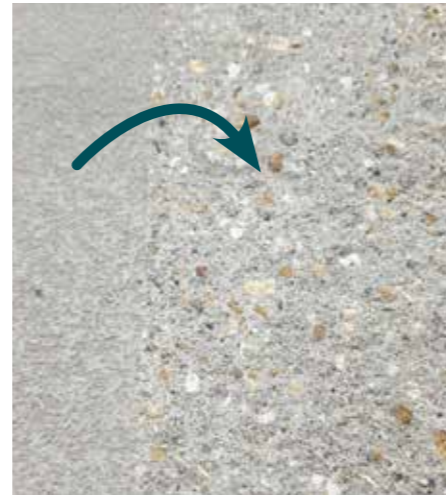
Concrete blasted, scarified, or grinded to an open texture exposed aggregate finish
