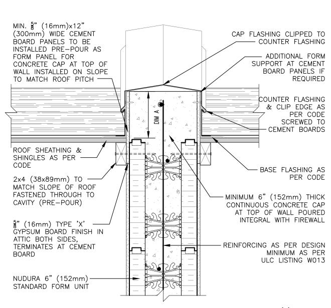
NOTE: DIMENSION 'A' MUST BE MINIMUM 6" (152mm) AS PER CODE FOR 2 HOUR FIREWALL (CANADIAN CODE)
