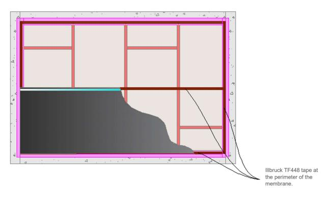
For low to medium wind loads the double sided tape should be applied around the entire perimeter of the membrane.
