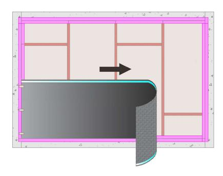
Unfurl the membrane horizontally and press the self adhesive strip on to the substrate ensuring that the membrane is applied smoothly and free from wrinkles and bubbles. Sections of masking tape can be applied on adhesive free edges if required to temporarily secure the membrane in position.
