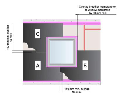
Horizontal overlaps are sealed with the self-adhesive bonding strips. Vertical overlaps are sealed with the correct illbruck tape, applied bubble and wrinkle free and all bonds are consolidated with a seam roller.
