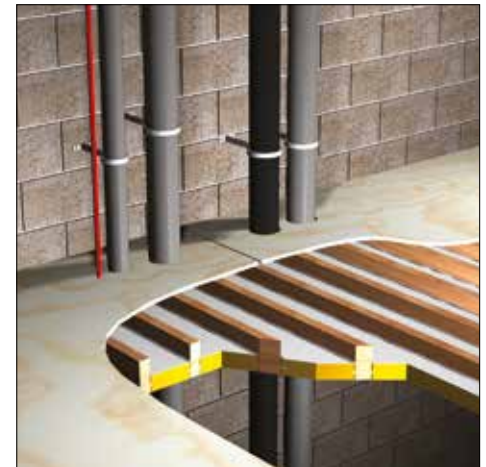
FB770 Intudeck between joists
