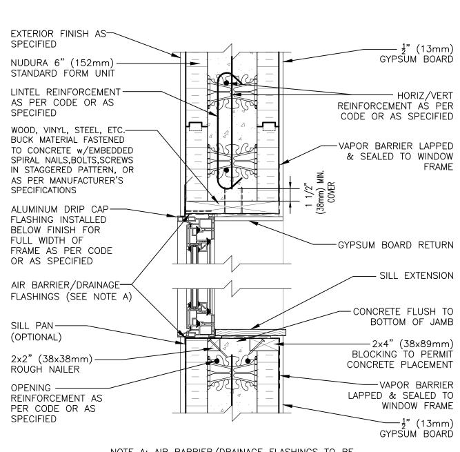
NOTE A: AIR BARRIER/DRAINAGE FLASHINGS TO BE INSTALLED AROUND COMPLETE OPENING PERIMETER AS PER SECTION 9.1 OF THE NUDURA INSTALLATION MANUAL OR AS DETAILED BY LOCAL APPLICABLE CODES (CODE GOVERNS)
