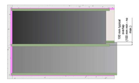
All vertical joints must be formed with a minimum 150 mm sealed overlap.
