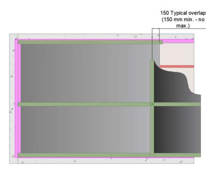
Once the joints have been formed and the membrane is temporarily secured, apply the correct illbruck tape to seal the overlap. The tape should be wrinkle and bubble free, and the bond consolidated with a seam roller.
