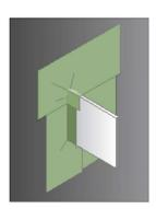
All incisions around any penetration are fully sealed with the correct illbruck tape.
