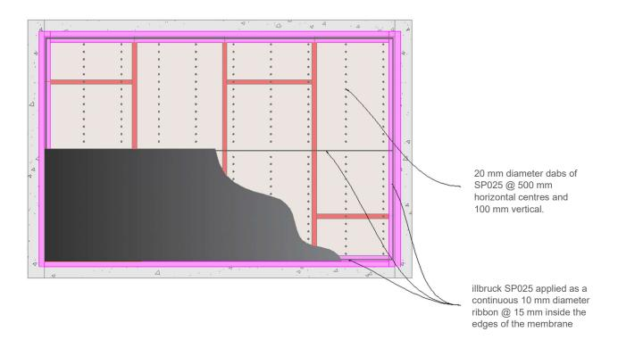
For low to medium wind loads a 10 mm diameter bead of SP025 adhesive should be applied around the entire perimeter of the membrane. For higher wind loads, the bond can be further enhanced by applying 20 mm diameter dabs of SP025 Fire Membrane Adhesive at 500 mm horizontal and 100 mm vertical centres.
