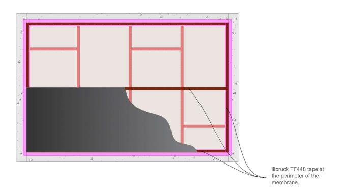
For low to medium wind loads the double sided tape should be applied around the entire perimeter of the membrane.
