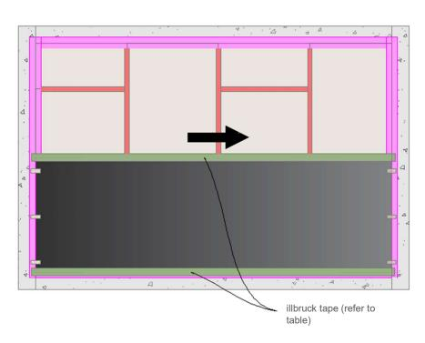
Unfurl the membrane horizontally until you have reached the end of the bay or an opening, applying more sections of masking tape at intervals of not less than 450 mm and not more than 1000 mm to temporarily secure the membrane in position.
