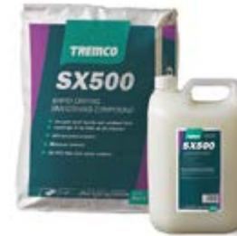
SX500 is a fast drying, smoothing compound for interior applications. It is moisture tolerant, has a 40% recycled content and can be applied in thicknesses of 2–15mm. SX500 has a compressive strength of 30 N/mm<sup>2</sup>. The product will accept foot traffic from as little as 30 minutes and some floor coverings from 90 minutes. With a 10-minute working time, SX500 is ideally suited to applications that require a same day turnaround.
